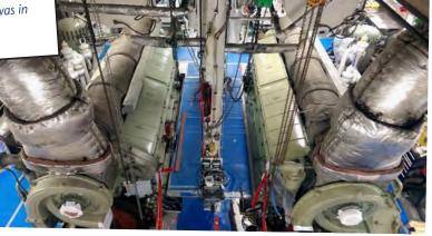
The Washington State Ferry MV KALEETAN in Seattle's Vigor Shipyard getting ready for a propulsion generator rebuild.
