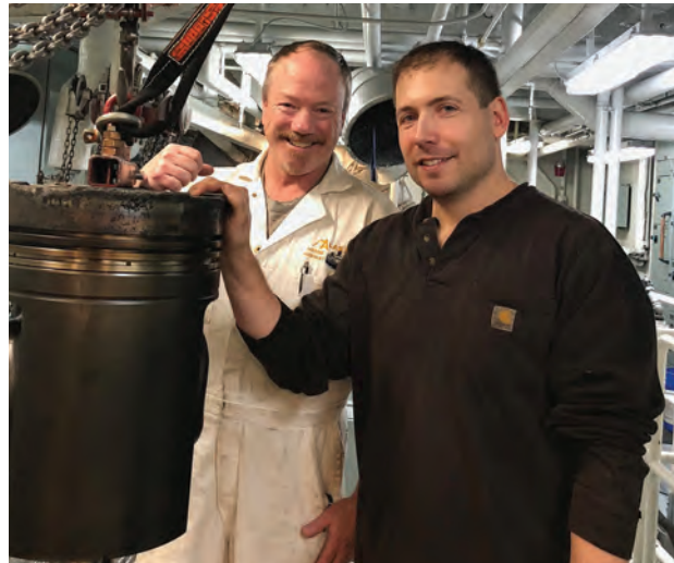
Chief Engineer Dominic Walsh and 1 st A/E Phil Brand pulling a piston aboard the Alaska Marine Highway System vessel M/V KENNICOTT. If the Governor's plan proceeds, the ferry system would operate only during the summer and signal an exodus of the experienced maritime workforce that keeps Alaskans safe and connected.
