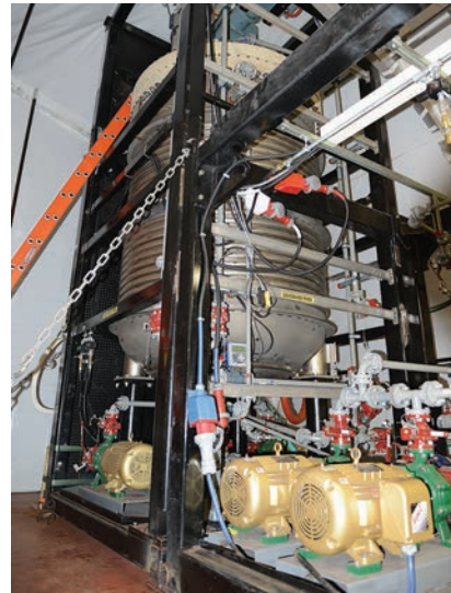
One of the two FDHS units installed on the CAPE RAY. Once the ship takes the chemical stockpile at Gioia Tauro, it will sail into the open Mediterranean before processing begins. The waste from the neutralized chemicals is set to go to land sites in Britain, Finland, Germany and Texas for ultimate disposal.
