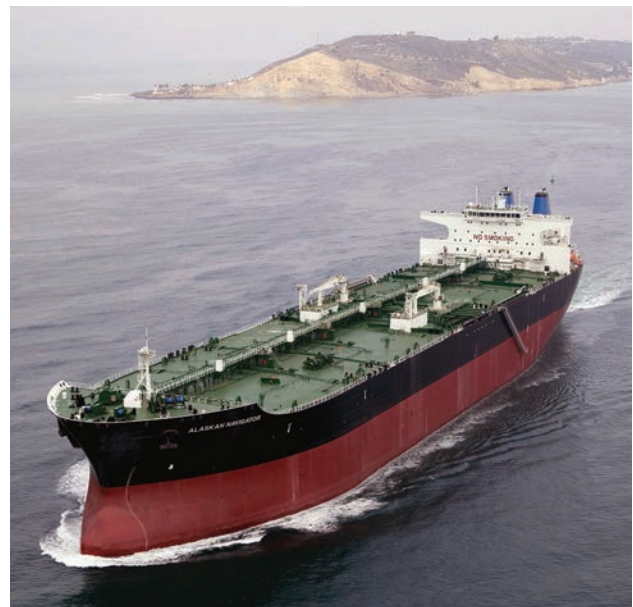
The double hulled Alaska class oil tanker ALASKAN NAVIGATOR operated by ATC. The vessel is 941 feet long with a capacity of 1.3 million barrels of crude oil.
