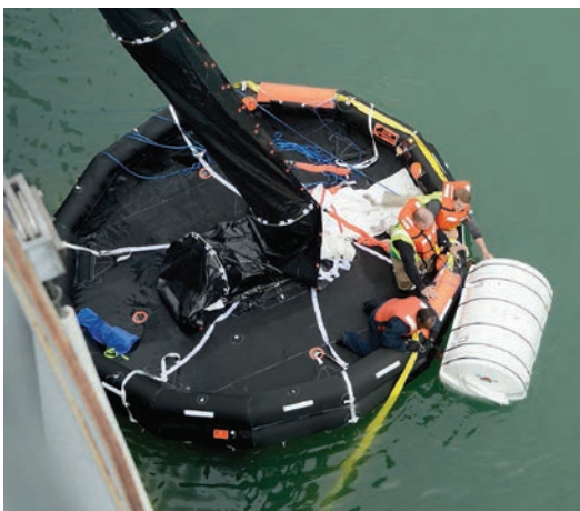
CAPE RAY crew secure the pod containing the life raft portion of the Marine Evacuation system to the base unit. The life-saving device has an escape chute where the crew could rapidly evacuate into a waiting life raft.
