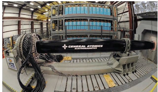
The U.S. Navy plans to install an electromagnetic railgun aboard the M.E.B.A.-crewed joint high speed vessel USNS MILLINOCKET in 2016. EM railgun technology uses an electromagnetic force - known as the Lorenz Force - to rapidly accelerate and launch a projectile at higher velocities than conventional guns.
