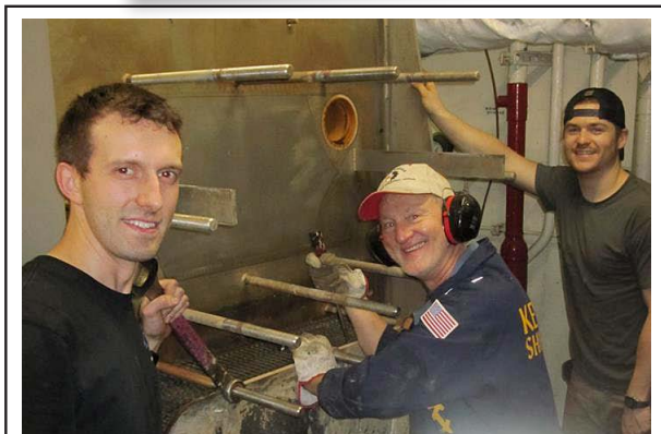
C/E Erik Barton took this shot of an evaporator overhaul onboard the SS SEAKAY SPIRIT. Making the magic happen (from left to right) are 1st A/E Phil Lessard, 3rd A/E Matt Burke and 3rd A/E Tim Martin.
