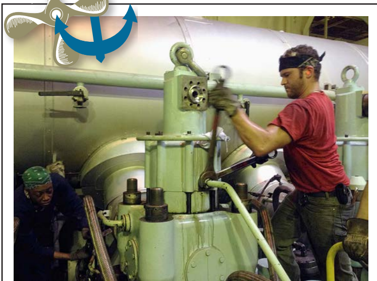
3rd A/E Yolanda Green (at left) and 2nd A/E Nate Gatchell working on the #6 exhaust valve aboard the CHARLESTON EXPRESS (Marine Transport Lines).
