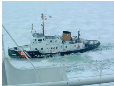
The U.S. Coast Guard vessel **MOBILE BAY** breaking ice to keep vessels on the move.
