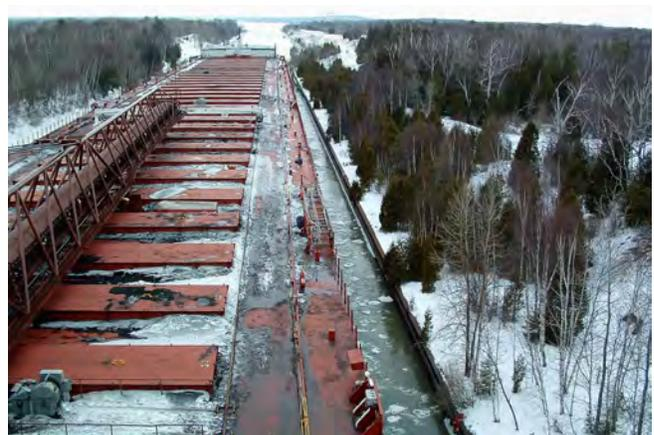
*Vessels on the Great Lakes maneuver through tight spaces such as the Sturgeon Bay Canal, which only allows for 20 feet of space on each side of the larger Lakers.*
