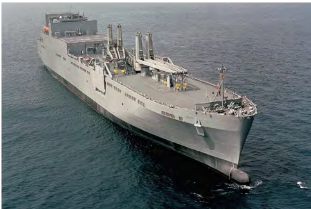
Military Sealift Command's USNS CHARLTON (T-AKR 314) is one of the eight Watson-class LMSRs. The LMSRs all have a commercial helicopter deck.
