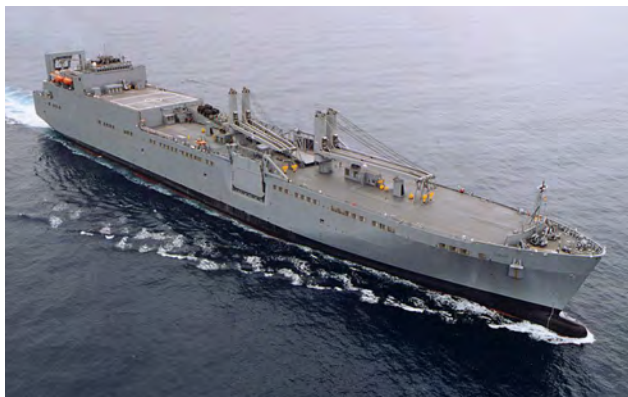
The USNS POMEROY (T-AKR 316) is one of the Watson Class vessels. Each of the ships have twin cranes allowing cargo to be loaded and unloaded.
