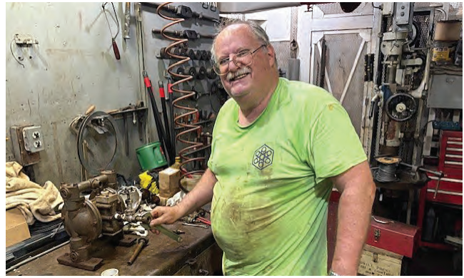
M.E.B.A. retired Chief Engineer Charles Norval volunteers his time to keep the Tampa-based floating museum ship SS AMERICAN VICTORY operational. The storied vessel served in World War II, Korea and Vietnam. Charles is seen here rebuilding a Wilden pump used to pump out the shaft alley.
