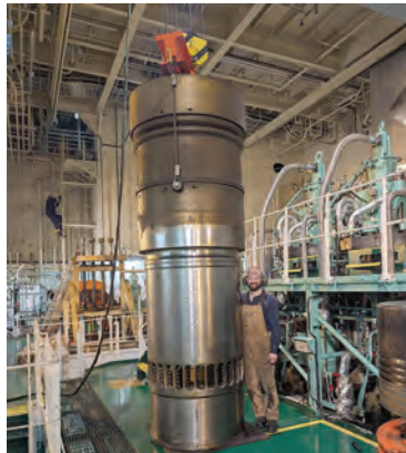
Alex Di Pietro doing a piston and liner pull on the (CMA CGM) APL PHOENIX in New Jersey recently. AMO & M.E.B.A. officers are crewing the vessel on a rotating basis in a special collaborative arrangement.
