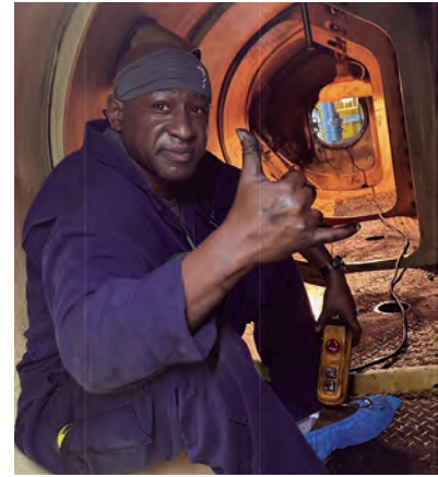
1st A/E Harry McKeever on the Matson LNG vessel MANUKAI doing a diesel engine scavenge air box inspection with C/E Tom Dewhirst.
