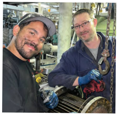
Onboard the Black Ball ferry MV COHO earlier this year, 2nd Engineer Nick Anderson and Oiler Gabriel Rosario overhauled the port main engine lube oil cooler during the annual dry dock in Ana-cortes. (Photo taken by COHO Chief Engineer Jess Johnson).
