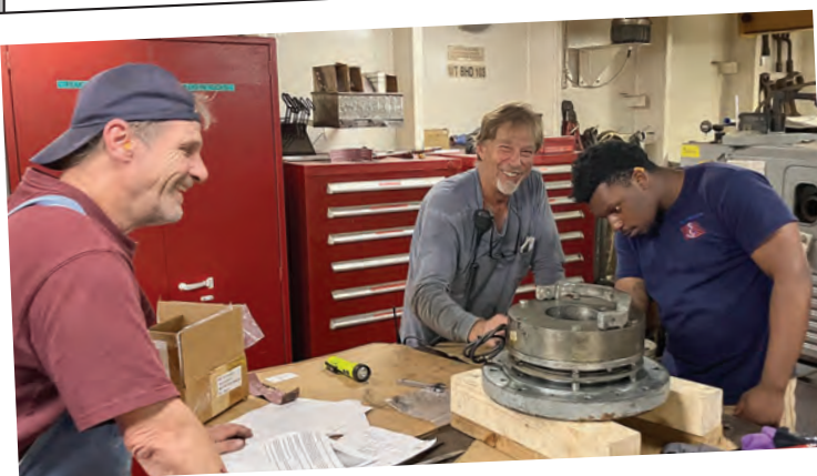
M.E.B.A. and MFOW aboard the Patriot-managed LMSR USNS POMEROY. Left to right are 2nd A/E Bobby Dance, Maintenance 1st Pat Barry and QMED D'Averyon Bloodworth repairing the brake on the ship's #5 mooring winch while in Baltimore, MD.
